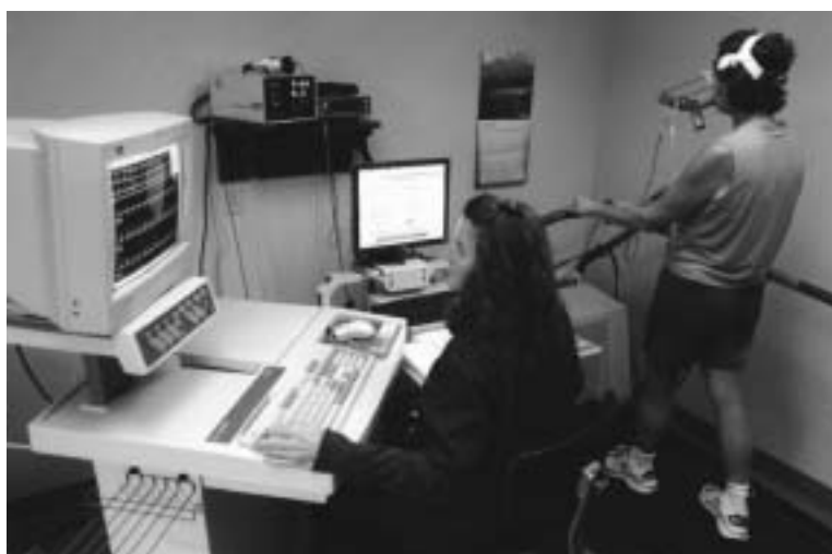
FIGURE 2. A patient undergoing a cardiopulmonary stress test. The head harness worn by the patient holds the mouthpiece and nonbreathing valve that is connected to a metabolic cart to the immediate left of the patient.
